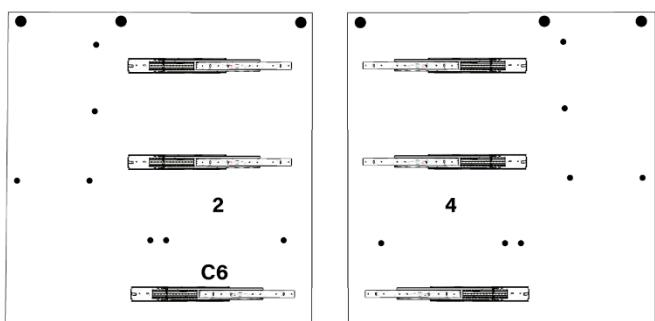
FIXAR CORREDIÇAS "C6" NAS LATERAIS "2" E "4" USANDO PARAFUSO "P1".
