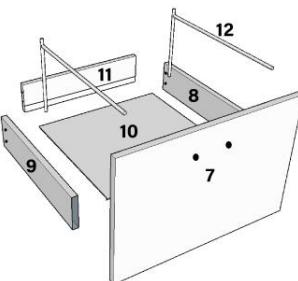
FIXAR CORREDIÇAS “C6” NA MARCAÇÃO DAS LATERAIS “8, 9” USANDO PARAFUSO “P1”.
