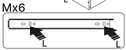
Coloque um parafuso L no furos indicados com
