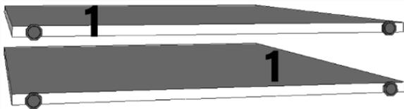
FIXAR A BUCHA DA SAPATA "B1" NAS FURAÇÕES DOS PÉS E DEPOIS APERTAR A SAPATA "S1".
