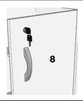
FIXAR FECHADURA "F2" + DISTANCIADOR "D1" NA PORTA "8" USANDO PARAFUSO 3,5X14 "P1".
