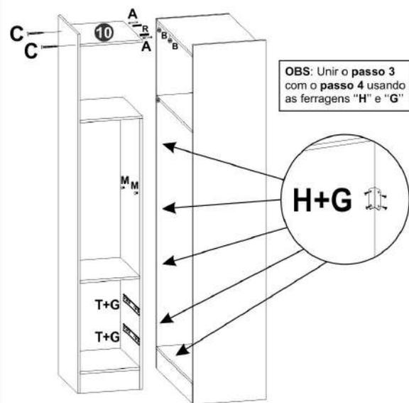
**OBS:** Unir o passo 3 com o passo 4 usando as ferragens "H" e "G"
