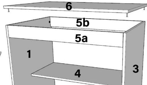
APÓS, ENCAIXE O TAMPO SOBRE AS LATERAIS "1 E 3". PARA FIXAR ELA, ENCAIXE NOS FUROS DAS LATERIAS O TAMBOR MINIFIX "M1" E APERTE-OS.
