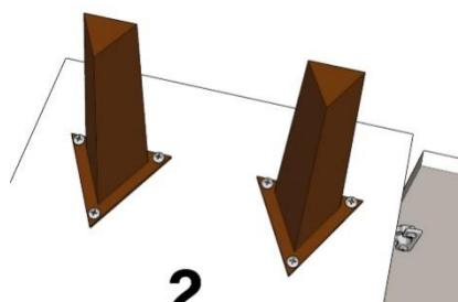
FIXAR PÉ TRIANGULAR "S2" NA BASE "2" USANDO PARAFUSO 3,5X14.
