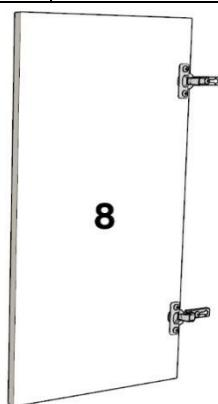
NA PORTA ESQ "8" FIXE A DOBRADIÇA BRAÇO CURVO "D1" USANDO PARAFUSO 3,5X14.
