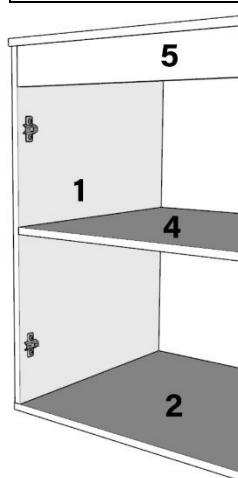
NA LATERAL "1" FIXE A DOBRADIÇA CALÇO "D3" USANDO PARAFUSO 3,5X14 "P1".
