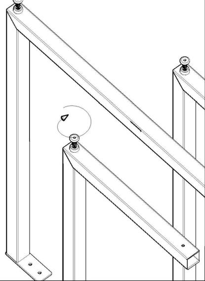
2º) PARAFUSE OS PÉS NA CHAPINHA DE UNIÃO (E) USANDO O PARAFUSO (D) UTILIZE A CHAVE ALLEN NO PROCESSO E APERTE.
