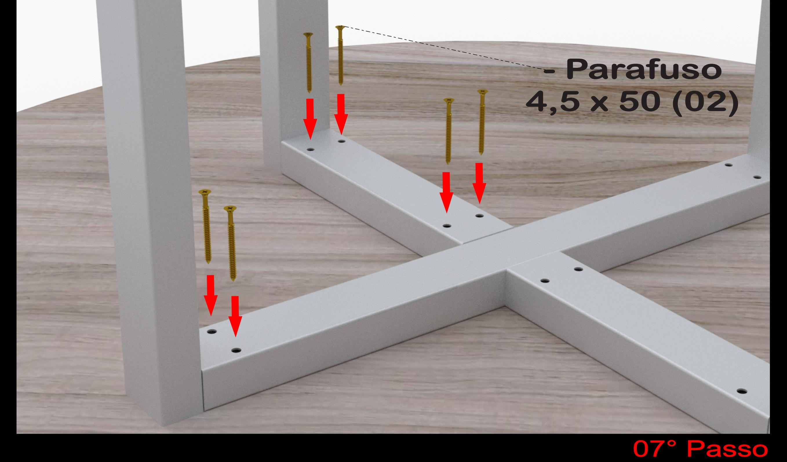
The image shows a white metal frame being assembled on a light-colored wooden surface. The frame consists of several L-shaped brackets. Red arrows point to the holes in the brackets where screws are being inserted. A dashed line points from the text to the top of the frame. The text indicates the type and quantity of screws to be used.
