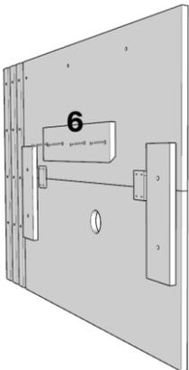
FIXAR TRAVESSA "6" NO PAINEL "1" UTILIZANDO PARAFUSOS "P2". ATENTE-SE QUE O CHANFRADO DEVE ESTAR PARA BAIXO. (CONFORME NA IMAGEM).
