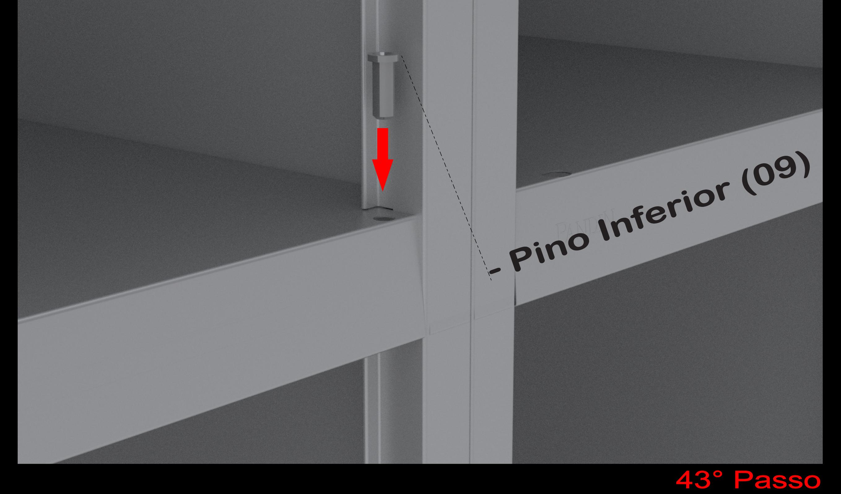
A technical diagram showing a window frame assembly step. A vertical metal pin is being inserted into a hole in a horizontal frame component. A red arrow points downwards from the top of the pin to the hole. A dashed line connects the top of the pin to a text label. The background shows a perspective view of the window frame with a dark grey interior and a light grey exterior.
