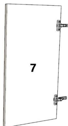
NA PORTA ESQ "7" FIXE A DOBRADIÇA BRAÇO CURVO "D1" USANDO PARAFUSO 3,5X14.
