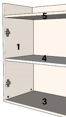
NA LATERAL "1" FIXE A DOBRADIÇA CALÇO "D3" USANDO PARAFUSO 3,5X14 "P1".
