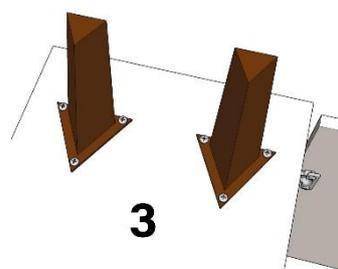
FIXAR PÉ TRIANGULAR "S2" NA BASE "3" USANDO PARAFUSO 3,5X14.
