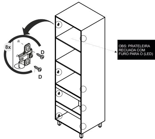
**08** Fixação das Portas
