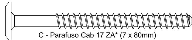
C - Parafuso Cab 17 ZA\* (7 x 80mm)
