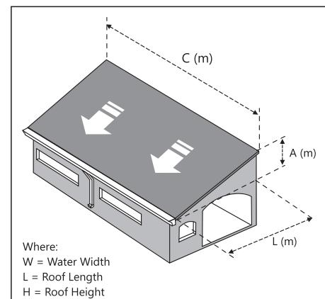
For roofs with inclination of 20°, the maximum area by nozzle (RMA) which gutter can exhaust on the main regions is given by the Pluviuometric Intensity (PI) calculation.
