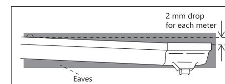
In this way, the outlet nozzles will be on the lowest point and no standing water will be inside the gutter.
