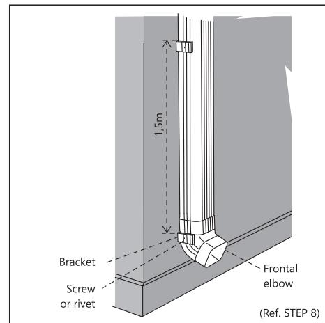
In case gutter system is assembled far from wall, attach a frontal elbow (CAL/JOF) on nozzle's exit, noting water flow direction indicated by an arrow on piece's lateral; next, cut a piece of conductor (CAL/CDT) sufficient to reach the wall, and attach elbow.
