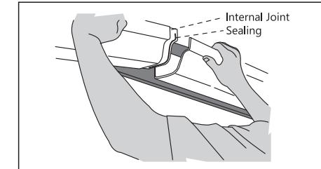
Make sure each sealing lace is in contact with each one of the pieces which are being united (gutter or miter).
