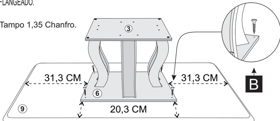
6º- CENTRALIZAR O TAMPO CONFORME MEDIDAS ABAIXO. FIXAR A BASE COM PARAFUSOS 04X25 FLANGEADO.
