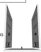
FIXAR CORREDIÇAS "C5" E "C6" NAS LATERAIS "2" E "4" USANDO PARAFUSO "P1".
