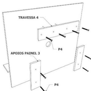
FIXAR TRAVESSA "4" NO PAINEL "1" (CHANFRO PARA DENTRO E PARA BAIXO COM PARAFUSOS "P2" (OS 2 FUROS CENTRAIS POSSUEM PRÉ MARCAÇÃO NO PAINEL).
