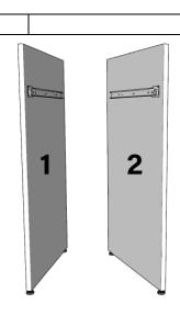
FIXAR A PARTE "1" DA CORREDIÇA "C5" NAS LATERAIS "1, 2" USANDO DOIS PARAFUSOS "P1" EM CADA LATERAL.
