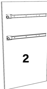
FIXAR A PARTE 1 DA CORREDIÇA "C5" NAS LATERAIS "1" E "2" USANDO DOIS PARAFUSOS "P1" EM CADA LATERAL, NAS DEVIDAS PRÉ-MARCAÇÕES EXISTENTES.
