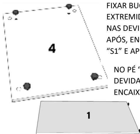
FIXAR BUCHA "B1" NAS 4 EXTREMIDADES DA BASE "4" NAS DEVIDAS FURAÇÕES. APÓS, ENCAIXE A SAPATA "S1" E APERTE-A.
