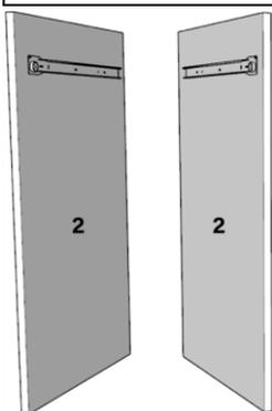
FIXAR A PARTE 1 DA CORREDIÇA "C5" NAS LATERAIS DOS PÉS "2" USANDO DOIS PARAFUSOS 3,5X14 "P1" EM CADA CORREDIÇA.
