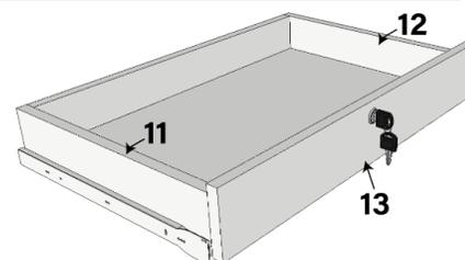
FIXAR A PARTE 2 DAS CORREDIÇAS "C4" USANDO DOIS PARAFUSOS "P1" EM CADA LATERAL "11" E "12".
