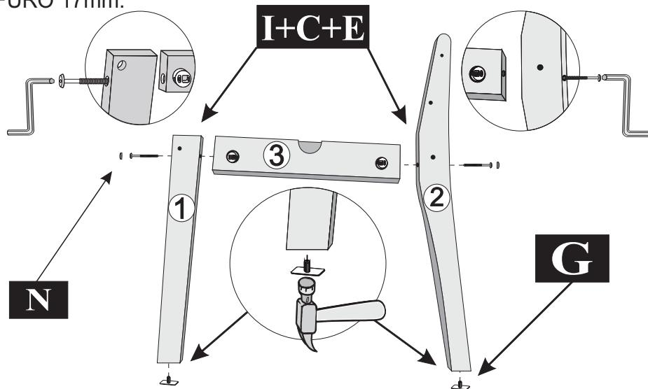
2º - UNIR O CONJUNTO LATERAL COM A TRAVA FRONTAL N°5 UTILIZANDO ANEL FIXADOR+PARAFUSOS 1/4X70+CHAVE ALLEN, UNIR TAMBÉM O CONJUNTO COM TRAVA DETALHE ENC. N°7 UTILIZANDO PARAF. 07x50mm CAB. 13 mm+CHAVE ZETA. EM SEGUIDA PARAFUSAR CHAPA 04 FUROS+PARAF. 3,5X12 UNINDO O PÉ TRASEIRO E A TRAVA.
