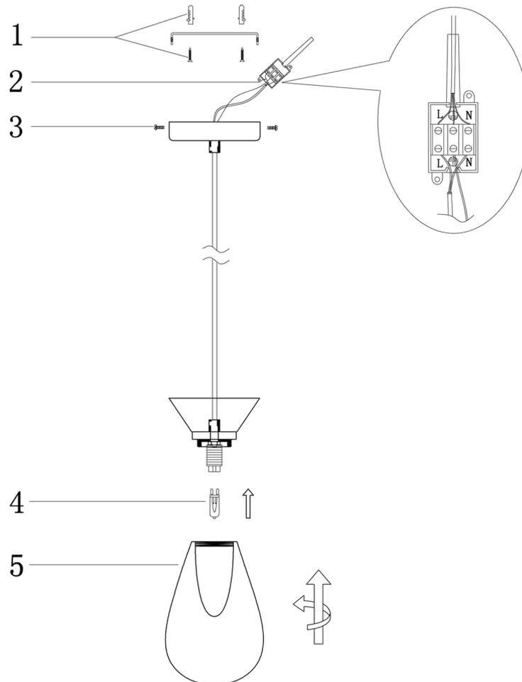
1. FIXE AS BUCHAS NA PAREDE E FIXE A ATRAVESSA COM AS BUCHAS NA PAREDE.
