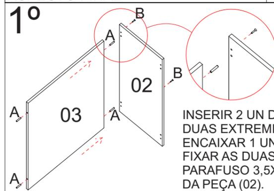
INSERIR 2 UN DA CAVILHA 6X30 (A) NAS DUAS EXTREMIDADES DA PEÇA (03) E ENCAIXAR 1 UN DA PEÇA (02). APÓS ISSO, FIXAR AS DUAS PEÇAS COM 02 UN DO PARAFUSO 3,5X40 (B) PELA FACE EXTERNA DA PEÇA (02).
