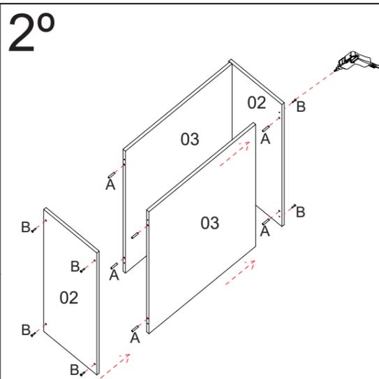
INSERIR 2 UN DA CAVILHA 6X30 (A) NA FACE DA PEÇA (02) QUE JÁ ESTÁ FIXADA E ENCAIXAR A OUTRA PEÇA (03). APÓS ISSO, INSERIR AS ÚLTIMAS 2 CAVILHAS (A) NA EXTREMIDADE DA PEÇA (03) E ENCAIXAR A LATERAL RESTANTE. POR FIM, FIXAR AS PEÇAS COM PARAFUSOS 3,5X40 (B) PELA FACE EXTERNA DAS PEÇAS (02).
