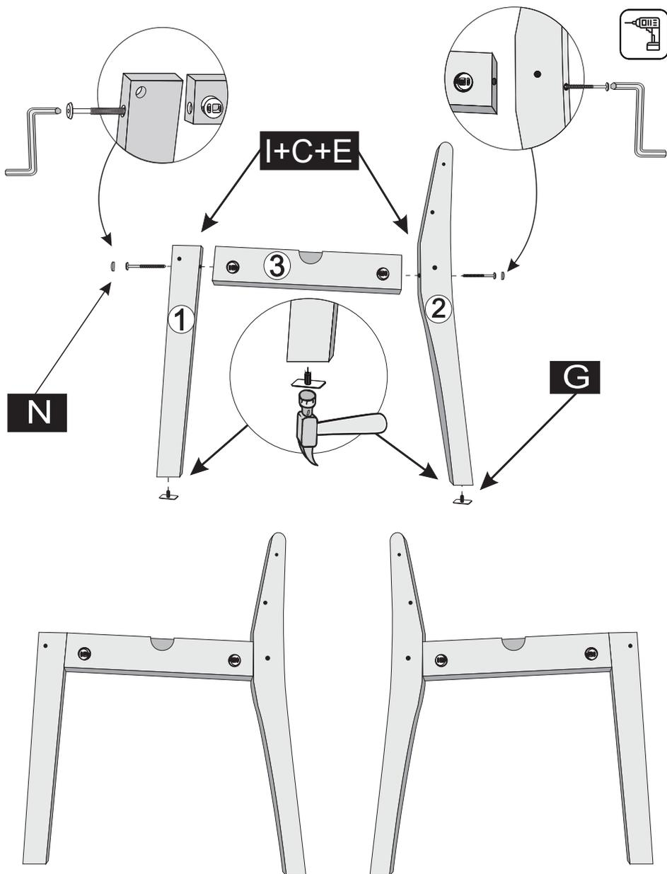
2º - UNIR O CONJUNTO LATERAL COM A TRAVA FRONTAL Nº5 UTILIZANDO ANEL FIXADOR+PARAFUSOS 1/4X70+CHAVE ALEN, UNIR TAMBÉM O CONJUNTO COM TRAVA DETALHE ENC. Nº7 UTILIZANDO PARAF. 07x50mm CAB. 13 mm+CHAVE ZETA. EM SEGUIDA PARAFUSAR CHAPA 04 FUROS+PARAF. 3,5X12 UNINDO O PÉ TRASEIRO E A TRAVA.
