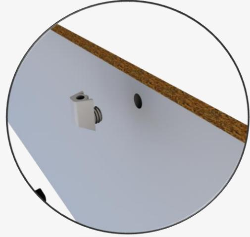
**4. POSICIONE O TAMPO (ITEM 1) EM UMA SUPERFÍCIE RETA E PARAFUSE A ESTRUTURA NO TAMPO UTILIZANDO OS LOCAIS INDICADOS, COM OS PARAFUSOS 4,8X13 (ITEM 7)**
