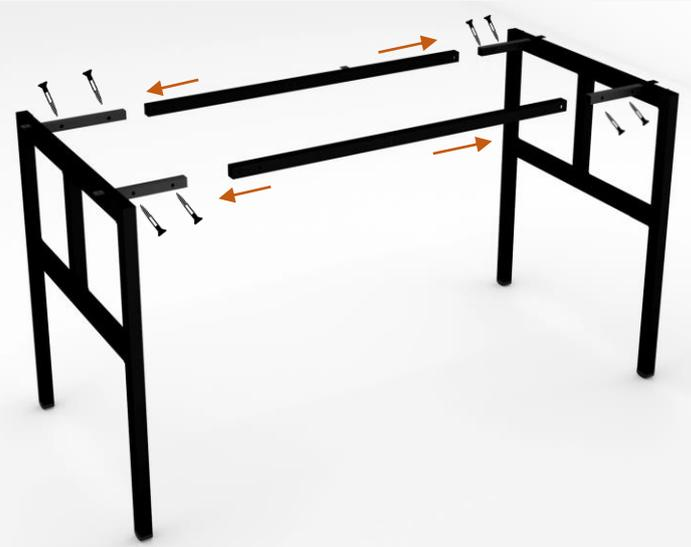
**3. COM A ESTRUTURA MONTADA, PARAFUSE A SAIA (ITEM 2) NAS LATERAIS DOS PÉS COM OS PARAFUSOS 7,0X60 (ITEM 6)**
