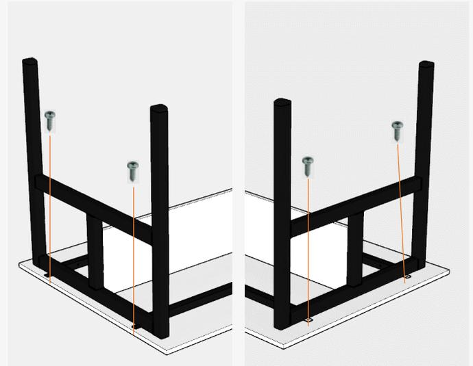
**6. PARA A MONTAGEM DOS BANCOS, BASTA PARAFUSAR A ESTRUTURA NOS TAMPOS COMO NA ETAPA 4 UTILIZANDO OS PARAFUSOS 4,8X13 (ITEM 7)**
