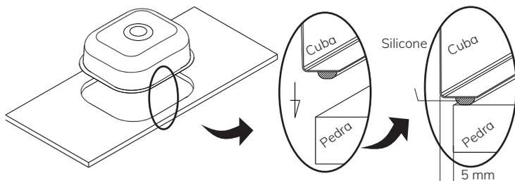
Important: The tub should be centered on the cut done previously with the help of the jig, note that it will have a recoil of 5mm between the stone and the radius, that will help in the hygiene of your sink, being easier to clean and prevent ingaccumulate summation of dirt under the stone.
