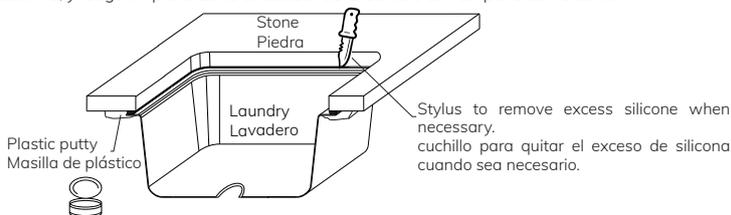
After fixing, check the need to remove excess silicone using a blade, then clean the region around the tank with a cloth with alcohol.
