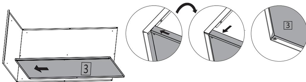
03 ENCAIXE A LATERAL NO FUNDO E NA COSTA, EM SEGUIDA APARAFUSE NOS PONTOS INDICADOS.
