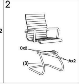
It is import to assemble all parts so that the directional "Arrows" point in the same direction. Make certain that all screws are FULLY tightened before using the chair. Each month check all screws and tighten and that may have loosened.
