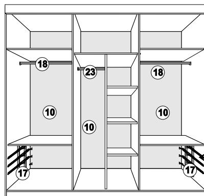
MONTAR O ALONGADOR (18) NA LATERAL COM PARAFUSO 7 X 35 (P8)
