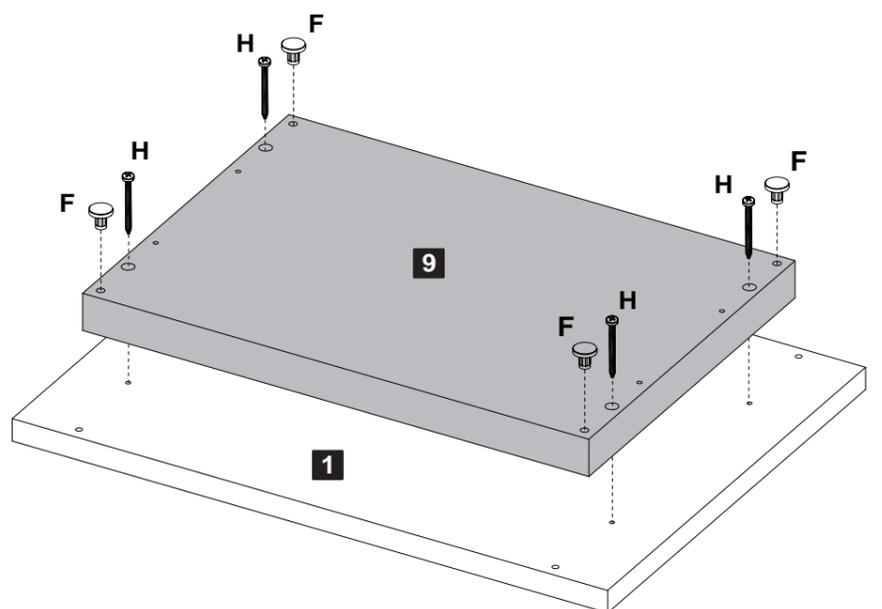
F Sapata Fixa Ø5x10mm 04 H Parafuso Ø3,5x30mm CP 04
