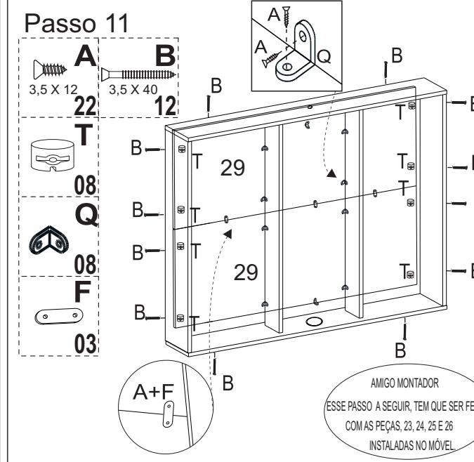
DEPOIS DE MONTADO A CAIXA NO PASSO ANTERIOR, FIXE A PARTE FRONTAL DO PAINEL.
