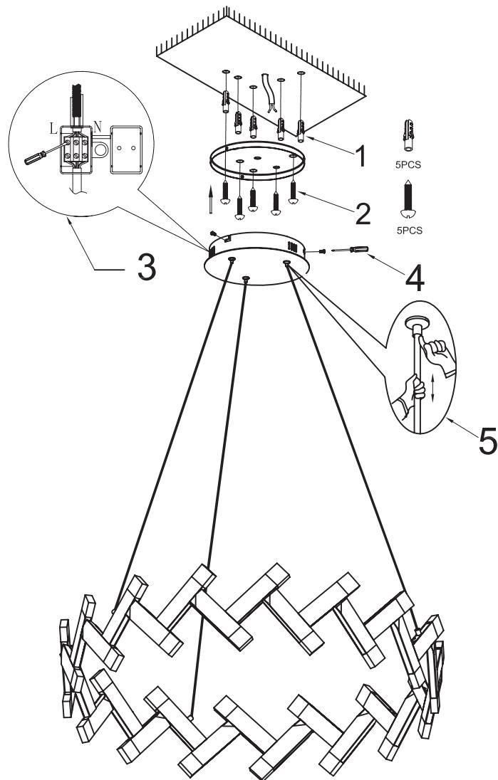
1. Insert the rubber plug into the ceiling
