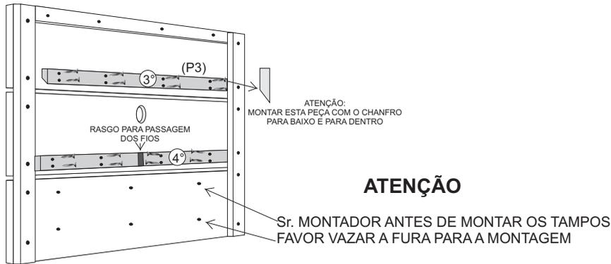
5° - MONTAR O TAMPO INFERIOR NO PAINEL COM PARAFUSO 5 X 40 (P4), PARAFUSANDO POR TRÁS.
