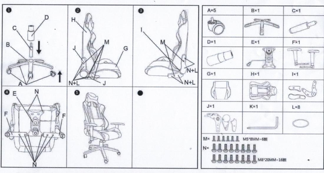
It is important to assemble all parts as the directional "ARROWS" point to. Make certain that all screws are fully tightened before using the chair, Each month check all screwsand tighten those that may have loosened. WARNING:Do not stand on the chair for any purpose
