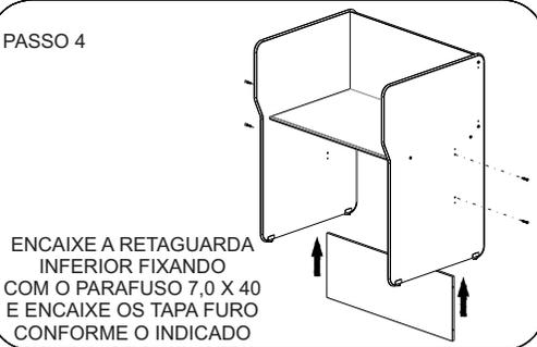
ENCAIXE A RETAGUARDA INFERIOR FIXANDO COM O PARAFUSO 7,0 X 40 E ENCAIXE OS TAPA FURO CONFORME O INDICADO
