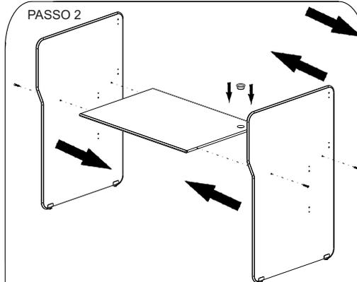
ENCAIXE O TAMPO FIXANDO COM O PARAFUSO 7,0 X 40 PRESSIONANDO AS LATERAIS UMA CONTRA A OUTRA CONFORME O INDICADO
