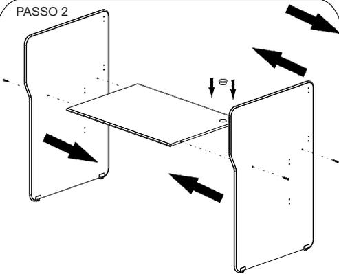
ENCAIXE O TAMPO FIXANDO COM O PARAFUSO 7,0 X 40 PRESSIONANDO AS LATERAIS UMA CONTRA A OUTRA CONFORME O INDICADO
