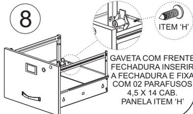
8 GAVETA COM FRENTE FECHADURA INSERIR A FECHADURA E FIXA COM 02 PARAFUSOS 4,5 X 14 CAB. PAINELA ITEM 'H'
