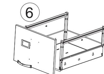
6 FIXE A FRENTE COM OS PARAFUSOS ITEM 'N', PUXADOR FIXAR COM OS PARAFUSOS ITEM 'L' E ENCAIXE O PORTA ETIQUETA
