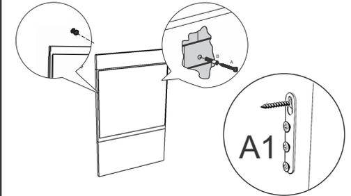
8.1: Fixe os parafusos ( M ) na parede com as buchas( L )
