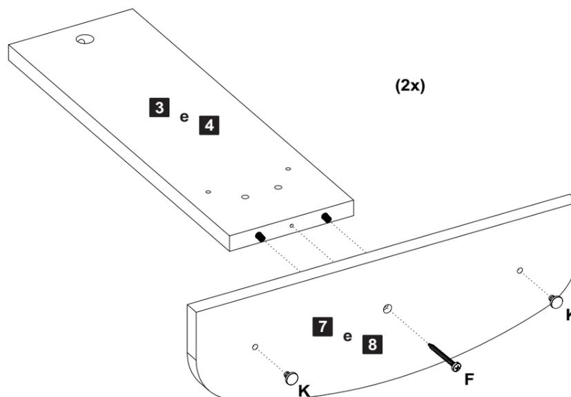
F Parafuso Ø3,5x40mm CP 02 K Sapata fixa Ø3x11mm 04
