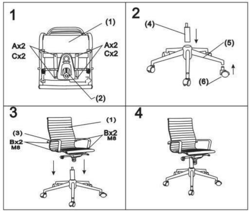
It is import to assemble all parts so that the directional "Arrows" point in the same direction. Make certain that all screws are FULLY tightened before using the chair. Each month check all screws and tighten and that may have loosened.
