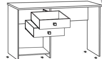
Posicionar as gavetas e ajustá-las, fixar as sapatas 15x15
