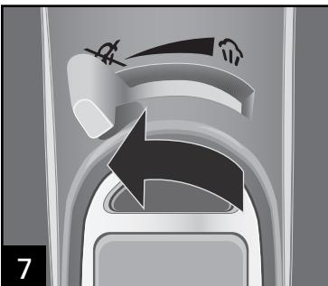
Para desligar o ferro, coloque a chave Ajuste do Vapor no
