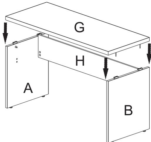
ENCAIXE O TAMPO ITEM 'G' NOS ESPAÇADORES ITEM 'J' FIXANDO COM OS PARAFUSOS MINIFIX ITEM 'I' E CAVILHA DE MADEIRA ITEM 'E' APERTE BEM
