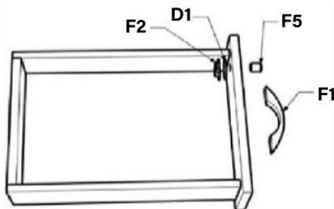
INSERIR DISTANCIADOR “D1” + FECHADURA “F2” NA PARTE INTERNA DA GAVETA.
