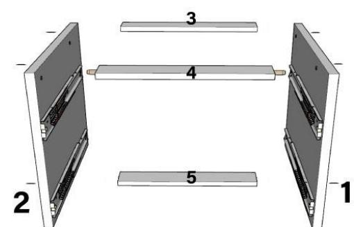
FIXAR AS TRAVESSAS “3, 4 E 5” COM OS PARAFUSOS “P3” NO EXTERNO DO GAVETEIRO.
