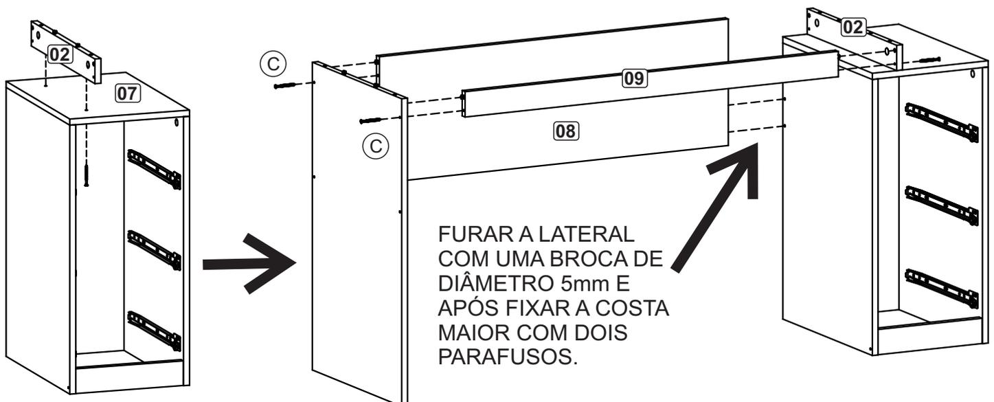
FURAR A LATERAL COM UMA BROCA DE DIÂMETRO 5mm E APÓS FIXAR A COSTA MAIOR COM DOIS PARAFUSOS.
