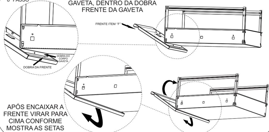
APÓS ENCAIXAR A FRENTE VIRAR PARA CIMA CONFORME MOSTRA AS SETAS
