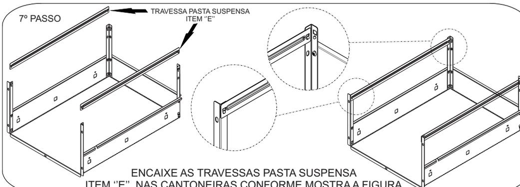
ENCAIXE AS TRAVESSAS PASTA SUSPensa ITEM "E", NAS CANTONEIRAS CONFORME MOSTRA A FIGURA
