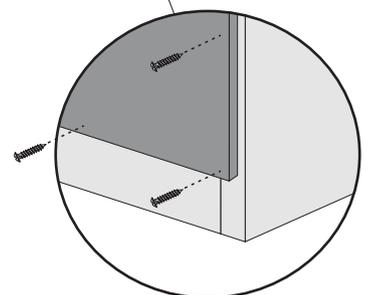
26 -FIXE OS CONECTORES (H) NAS LATERAIS (01) E ( 02 ) COM PARAFUSO (D)
