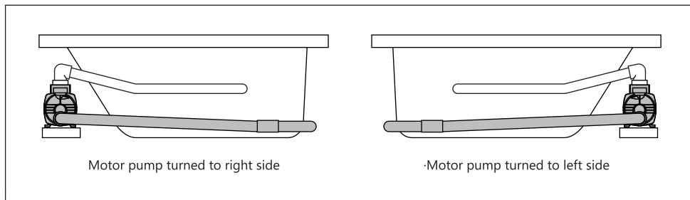
The suction pipeline can be assembled with motor pump turn to right or left side (picture above), according to the need, and in a manner which the motor pump is turned to the inspection door to facilitate use and maintenance.
