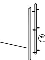
MONTAR O ALONGADOR (18) NA LATERAL COM PARAFUSO 7 X 35 (P8)
