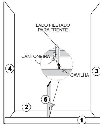
MONTAR A BASE DO ARMÁRIO (06) NAS LATERAIS (03) E (04) COM O PARAFUSO 5,0 X 4,0 (P4) E NA DIVISÃO DA SAPATEIRA (05) COM CAVILHA 6 X 45 (C3)
