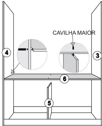
MONTAR A DIVISÃO DO ARMÁRIO (07) NAS CAVILHAS (C3) JÁ MONTADAS NA BASE (06). MONTAR A PRATELEIRA (08) NA DIVISÃO (07) COM O PARAFUSO 5,0 X 4,0 (P4)
