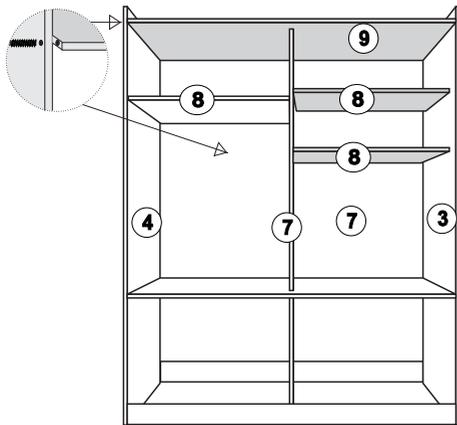
MONTAR AS CORREDIÇAS COM PARAFUSO 6 X 8 (P7) MONTAR A MOLDURA (11) COM O PARAFUSO 3,5 X 3,0 (P2) PARAFUSANDO DE BAIXO PARA CIMA. MONTAR O TRILHO COM PARAFUSO 3,5 X 14 (P1)
