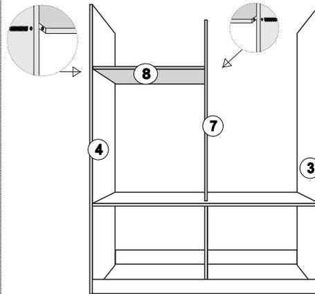
MONTAR O TAMPO (09) COM CAVILHA 6 X 30 (C2) NAS DIVISÕES (07) E COM O PARAFUSO 5,0 X 4,0 (P4) NAS LATERAIS (03) E (04) MONTAR AS OUTRAS PRATELEIRAS (08) E COM O PARAFUSO 5,0 X 4,0 (P4) NAS LATERAIS (03) E (04)
